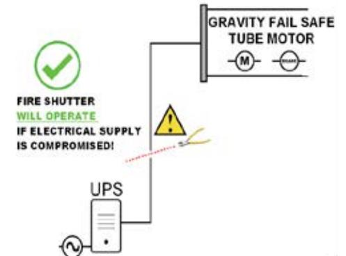
The Gravity Fail-safe motor has been tested and successfully passed to **BS EN 1634-1** at WarringtonFire. Under current regulations **BS EN 16034**, this motor can only be included within a fire shutter/fire curtain that has been tested with that motor type.
